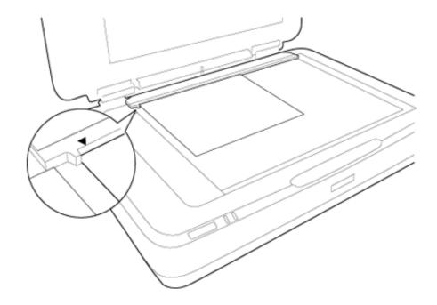
If the reflective document mat is installed in the Transparency Unit, remove it. Close the Transparency Unit.
