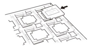
Place the slide holder on the scanner glass. Align the slide holder with the notch on the transparency guide, as shown below.
