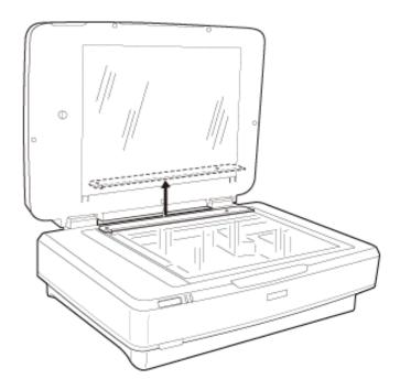
Slide the mat into the upper side, and then insert the tabs into the slots on the lower side slots on the Transparency Unit.
