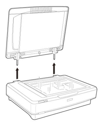
Align the pins of the unit with the holes of the scanner, and then lower the Transparency Unit until it rests securely on the scanner with the pins in the holes.
