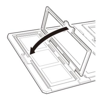
Place the film holder on the scanner glass and align it with the notch on the transparency guide, as shown below.
