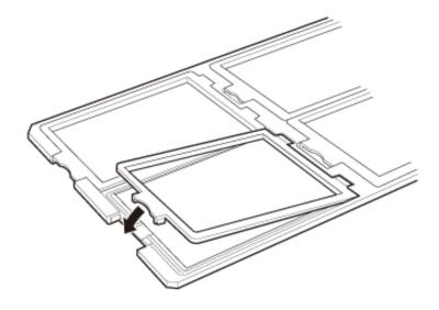
Place the holder on the scanner glass and align it with the notch on the transparency guide, as shown below.
