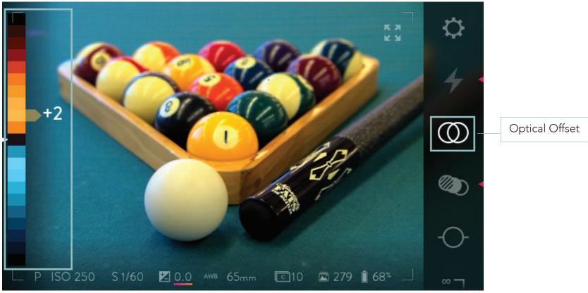
Rotate the front dial to adjust the optical offset.
