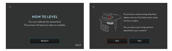
Follow the on-screen guide to calibrate the ILLUM level. You must remove the ILLUM lens hood and camera strap before calibrating. If you have attached the Lytro strap anchors to the ILLUM, click YES when prompted. If you have not attcahed the Lytro strap anchors, click NO. The 6 step calibration processis ready to start.
