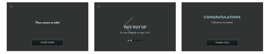
Place the ILLUM on a flat, level surface like a table. Touch the Start Now button on the screen. As prompted, rotate the ILLUM in the direction indicated by the arrow and place the ILLUM on that same flat table surface. You will be instructed to rotate and replace the ILLUM in the new orientation six times to complete the process. If you rotate the camera the wrong direction or skip a step when instructed, the calibration process will not complete.
