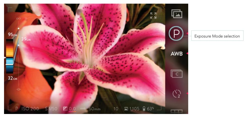
Tap the current exposure mode icon to open the submenu displaying the four options.
