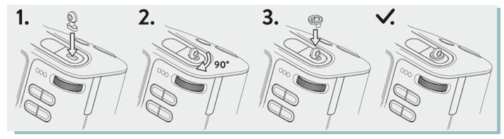
Once strap anchors are installed, attach the strap using the split-rings.
