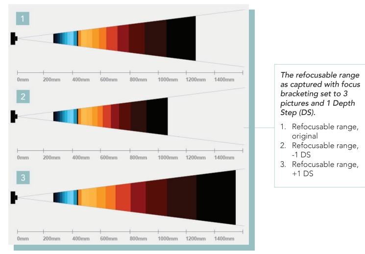
To use focus bracketing, add it to the Menu Bar (see Rearrange Menu). Then activate it and set the number of pictures that will be taken and the number of Depth Steps between each picture. For help setting those parameters, see Applying focus bracketing.
